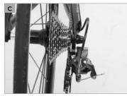
3. Check whether the chain still runs on the chainrings and the sprockets. If your SCOTT bike fell over to the chain side, verify the proper functioning of the gears. Ask somebody to lift your SCOTT bike by the saddle and carefully shift through all the gears. Pay particular attention when switching to the small gears, making sure the rear derailleur does not get too close to the spokes as the chain climbs onto the larger sprockets (c+d).
