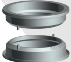
Headset indication and orientation, it is important to have the headset installed correctly depending on the setup. There are two types, 0° and 0.6°, these can be identified from the stamp on the inner surface of the headset cup.
