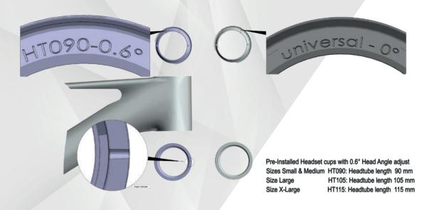
For 0.6° this can be installed at + or - but it is essential that the angle indication markers on the headset are set opposite to each other, top facing forward and bottom facing backwards (or vice versa).
