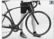
6. Finally, take a good look at the whole SCOTT bike to detect any deformations, colour changes or cracks. Ride back very carefully by taking the shortest route possible.
