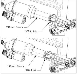
Figure 3 - Shock and Shock Link Configurations
