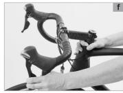
To check whether the headset runs smoothly, lift the frame up until the front wheel no longer touches the ground. The handlebars should turn from far left to far right without feeling roughness or tightness at any point. With a gentle tap on the handlebars the fork should turn easily from the middle position (a).
