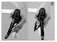
The shifters are positioned and actuated like the mechanical gears: With a Di2 you must only press control buttons, instead of pressing the entire brake lever or the lever positioned behind inward as is the case with usual dual control shifters from Shimano. Shift to the larger sprockets by pressing the long control button on the side of the brake lever. When you press the triangular control button that is behind the brake lever the chain moves onto the smaller cogwheels.
