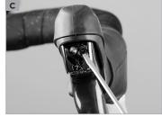
In the case of **SRAM** start by setting the cam disc on the slightly pulled and inward moved shifters. Screw in the screw positioned behind the hood in the body by using an Allen key **(e)**.
