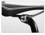
If you have a **single bolt system (c)**, the seat post for most of the sports saddles is designed for a saddle rail diameter of 7 mm.
