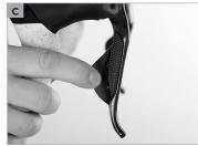
Depending on the gear system, gear shifting is initiated by actuating a brake lever/shifter unit **(c)** or a shifter **(d)** in the case of flat bars. Continue pedalling during gear shifting, however, at reduced pedalling force.
