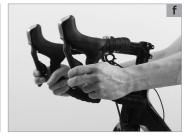
With disc brakes **(a)** you should have a stable pressure point at once. If you have to actuate the brake lever more than once to get a positive braking response, have the SCOTT bike checked by your SCOTT dealer immediately. For more information see the chapter "Brakes" and the manuals of the component manufacturers.
