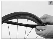
In the case of double wall rims the tape must cover the entire rim base, but it should not be so broad as to stand up along the inside edges of the rim trough. Rim tapes for this type of rim should only be made of fabric or durable plastic. If you are in doubt or if you have any questions, contact your SCOTT dealer.
