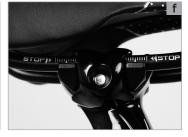
Position the saddle so that its upper surface is parallel to the ground. Tighten the bolt gradually and make sure
