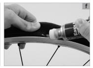
The first air blast is crucial for the mounting (a). The tyre must inflate and be in contact with the rim immediately to make sure no air escapes. It is therefore recommended that you use a compressor or a powerful track pump. Inflate the tyre with quick blasts.
