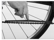
Replacing these components is relatively expensive compared with the costs of a new chain. It is therefore advisable to check the condition of the chain at regular intervals.
