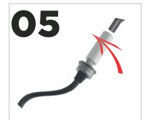
Unscrew the upper shock pump head from the shock valve.
