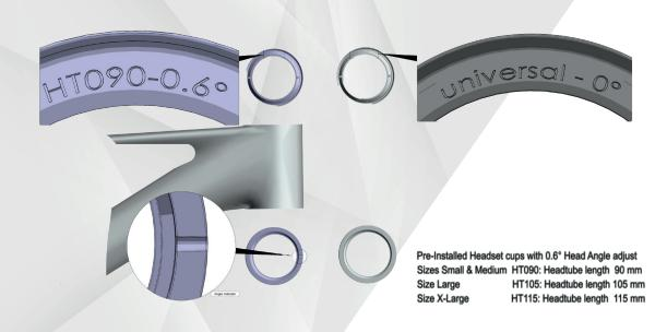
For 0.6° this can be installed at + or - but it is essential that the angle indication markers on the headset are set opposite to each other, top facing forward and bottom facing backwards (or vice versa).
