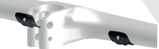
Please be aware that the maximum bolt length for the bottle cage on the seat tube is 10mm. The rivet nuts have closed ends, and using a longer bolt may result in damage to the frame.
