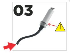
Make sure there is no gap between the two shock pump heads. Then pump the air to the required pressure.
