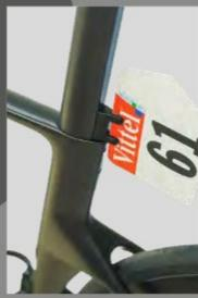
In the creation of the Teammachine R, no detail was overlooked, no matter how small. An example of this is the purpose-built Race Number holder. Seamlessly integrated into the seatpost, this design innovation eliminates the need for glue or zip ties, reflecting our commitment to both aesthetics, functionality and of course, racing.
