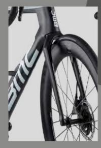
The ultrawide parallel fork legs are unlike anything else in the peloton. When rotating at speed, the front wheel produces a significant amount of turbulent air. We increased the inner fork spacing to allow that turbulent air to be shuttered away from the frame and reduce aero stall. The result is cleaner air that hugs the frame longer resulting in a significant drag reduction.
