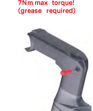
Install stem steerer clamp bolt - grease required!
