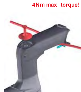
Install top cap and compression bolt
