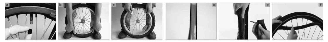
To make sure the inner tube does not get pinched between the rim and the bead, move the tyre sideways back and forth between the sides of the rim. While doing so, also check whether the rim tape has shifted.
