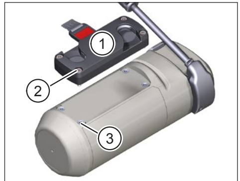
Fig. 3: Fasten FIDLOCK® Force Connector to Range Extender
