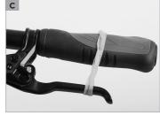
Be sure to transport your SCOTT bike only with the wheels mounted. If transporting your SCOTT bike with the wheels removed, make sure to mount the safety locks. Pull the brake levers and secure them with a strong elastic strap (c) when transporting a SCOTT bike with hydraulic disc brakes (d). This will prevent air from entering the system.
