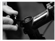
If you want to turn the stem around, you have to also release the bolts of the faceplate securing the handlebars (d). If the stem is fitted with a cap, you can simply take out the handlebars at this point. If it is not fitted with a cap, you have to remove the handlebar fittings.
