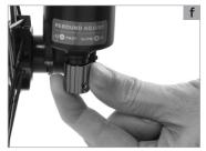
The typical setting of the rebound damping is an extension of the suspension components at reduced speed, however not at a sluggish pace. A rebound movement at reduced speed ending up in a sluggish movement is definitely a too high damping.
