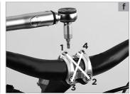
Check whether the back of your hand forms a straight line with the line of your forearm (a). Retighten the units with a torque wrench and do a twist test! The brake levers need not be absolutely tight. In case of a fall it is an advantage when the brake levers can be turned.
